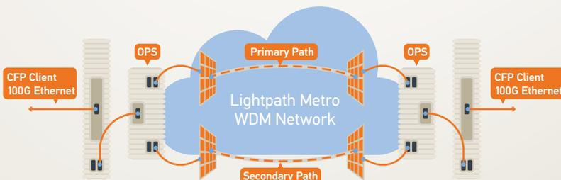
**Path Protection:** An Optical Protection Switch (OPS) is the protection mechanism that will provide a sub-50 ms protection switch.
